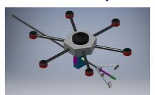
The radiation monitor robot monitoring the storage of containers with uranium hexafluoride in the open air
